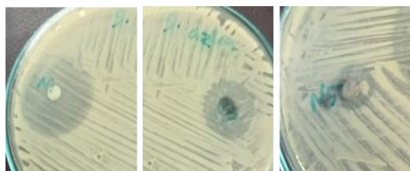
Fig.7. Activity of a) \text{NiFe}_2\text{O}_4 b) \text{NiCr}_{0.5}\text{Fe}_{1.5}\text{O}_4 and c) \text{NiCrFeO}_4 against S-aureus
