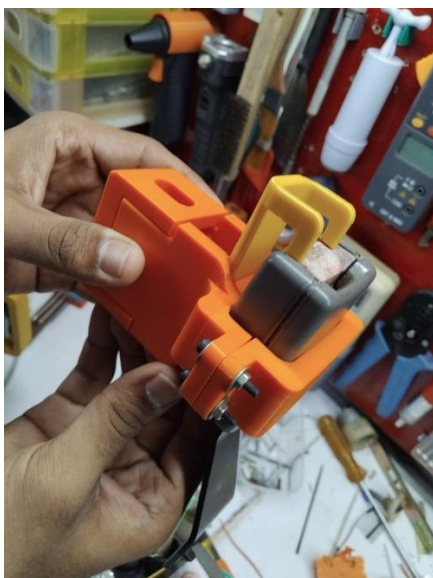
Fig. 4. Seatbelt unlocking mechanism
