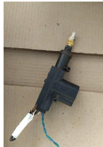
Fig. 5. Door Unlocking Linear Actuator
