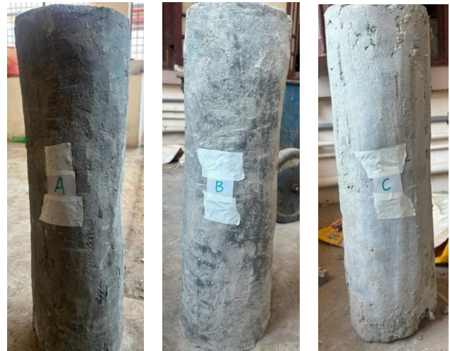
Fig. 8. Group B- Columns Retrofitted with 0.5% PVA Powder Mortar Mix
