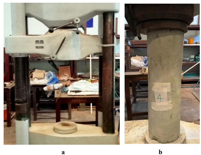
Fig. 9 (a) Universal Testing Machine (b) Test Setup of Sample Column
