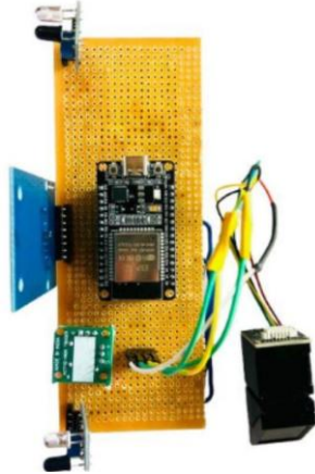
Fig. 5. Assembled hardware prototype showing ESP32, fingerprint sensor, RFID reader, and IR sensors on a common perf-board
